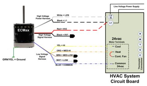
**Rotation** is determined automatically the first time the motor is operated. It is important to operate the motor for the first time in the HVAC system. Do not bench test the motor. The first time the motor is operated the following sequence should be recognized:
